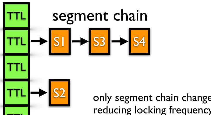
only segment chain changes need locking: reducing locking frequency by 10,000s times
